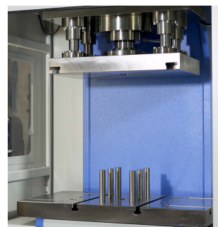
Lower hydraulic cushion and ejector
